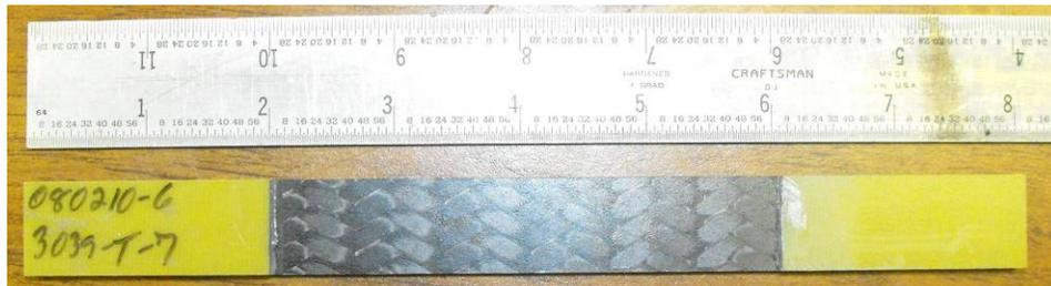
**Figure 12. Modified ASTM D 3039 Transverse Tensile**
