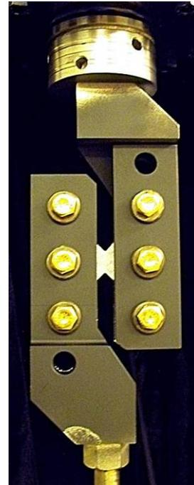
**Figure 23. Transverse Shear Setup**
