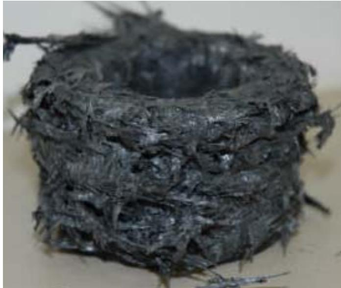
Figure 4.23: Failure mode produced during crush testing of TFO-2.
