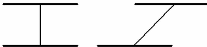
Figure 6.9. A schematic of a beam element connecting two shells in the undeformed (left) and deformed (right) positions demonstrating the beam elongation that occurs under pure shear loading.
