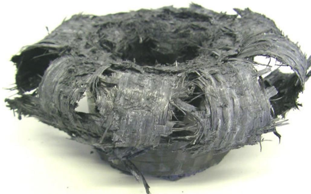
Figure 4.9. Example of the splaying mode of failure observed experimentally produced by Toray 5-harness satin weave.
