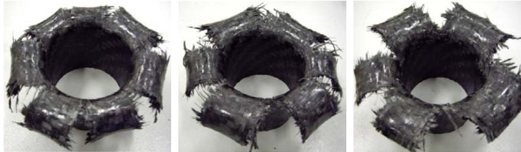
Figure 4.20. Images of the tubes crushed on (L-R) 5mm, 7.5mm and 10mm plug initiators showing the increased curvature of the fronds for the reducing plug radius.
