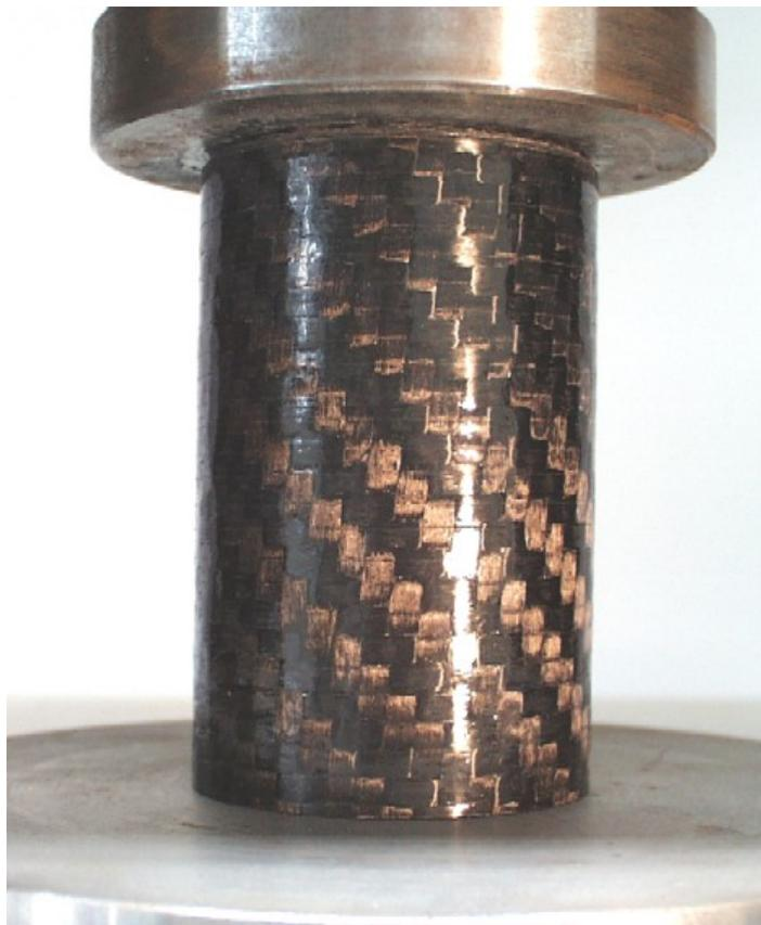
Figure 4.15. An example of the surface finish produced from shrink tape application.
