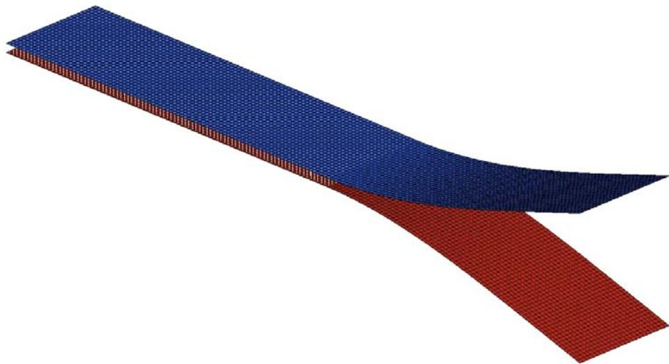
Figure 6.3. Image of CFRM DCB simulation underway.
