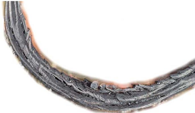
Figure 7.19. Image of experimental crush-zone produced from Toray tube crushed on a 5mm plug-initiator.
