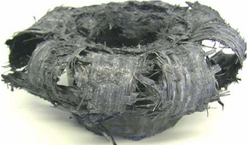
Figure 2.13. A crushed carbon/epoxy tube clearly showing the fronds, separated by axial tears and the ring of debris on the upper surface. (photo taken by M.Silcock)
