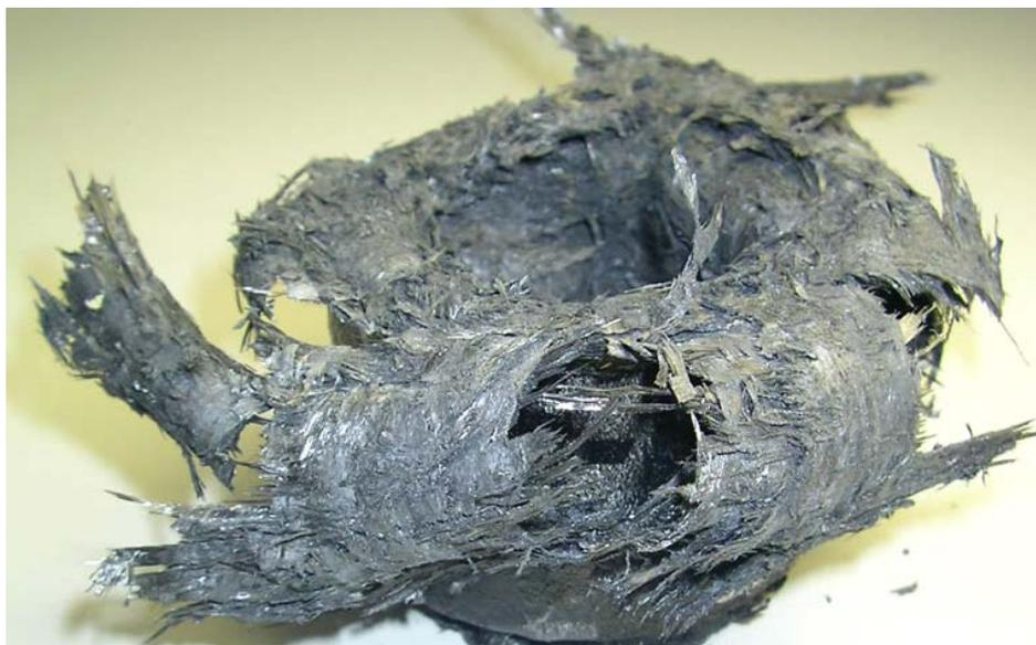
Figure 4.26. Image of a 2x2 twill Toray tube crushed on a flat-platen showing a variation in the failure mode with some transverse shearing.
