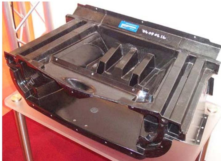
Figure 2.6. Lotus Elise composite crush box. (photo taken by M.Silcock at JEC Expo, Paris, 2005)
