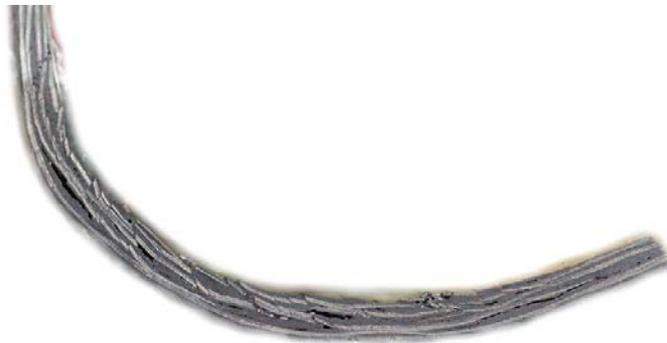
Figure 7.24. Image of experimental crush-zone produced from Toray tube crushed on a 7.5mm plug-initiator.
