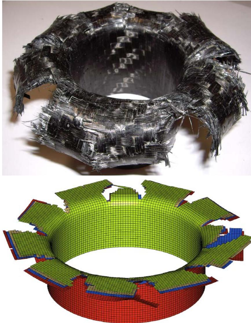
Figure 7.21. Images of experimental (above) and simulated (below) Toray tubes crushed on 5mm plug initiator.
