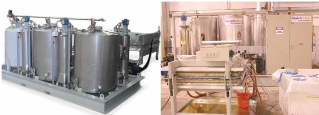
Figure 2.24. Left: Image of backside of QS plant showing the three fluid storage tanks with the cure chamber in the background. Right: Front side of QS plant showing the clamshell cure chamber in the foreground. (photos taken by M.Herring, 2006)
