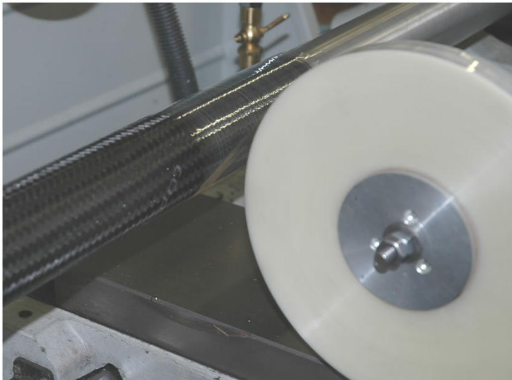
Figure 4.5. Close-up of shrink-tape application showing shrink tape roll holder and tensioning system.
