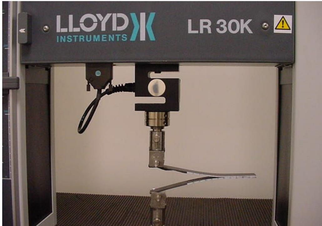
Figure 3.13. DCB test in progress on the Lloyd testing frame.
