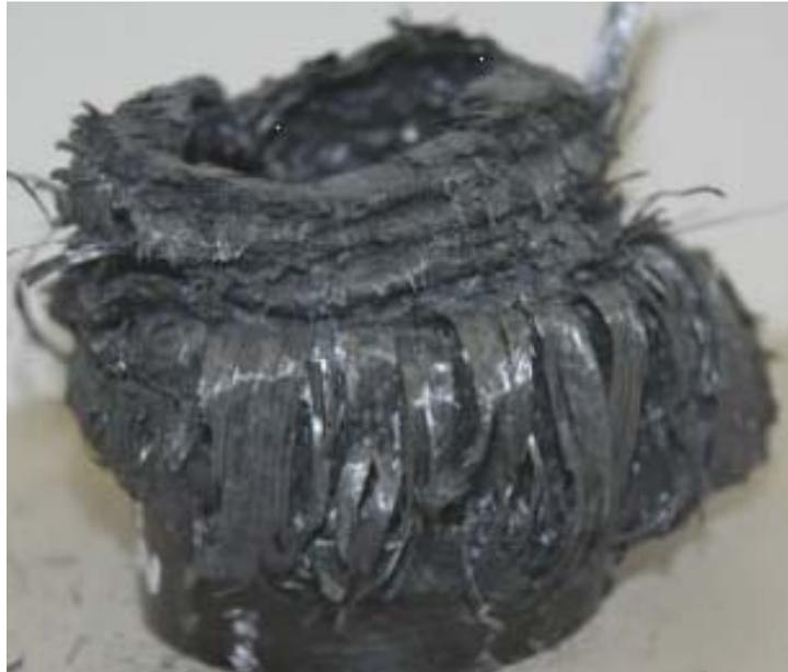
Figure 4.24. Failure mode observed in TFO-3 showing external fronds and internal concertina buckling.
