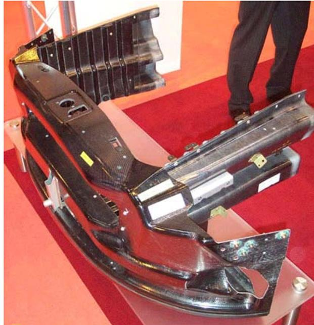
Figure 2.7. Aston Martin Vanquish composite crash structure. (photo taken by M.Silcock at JEC Expo, Paris, 2005)
