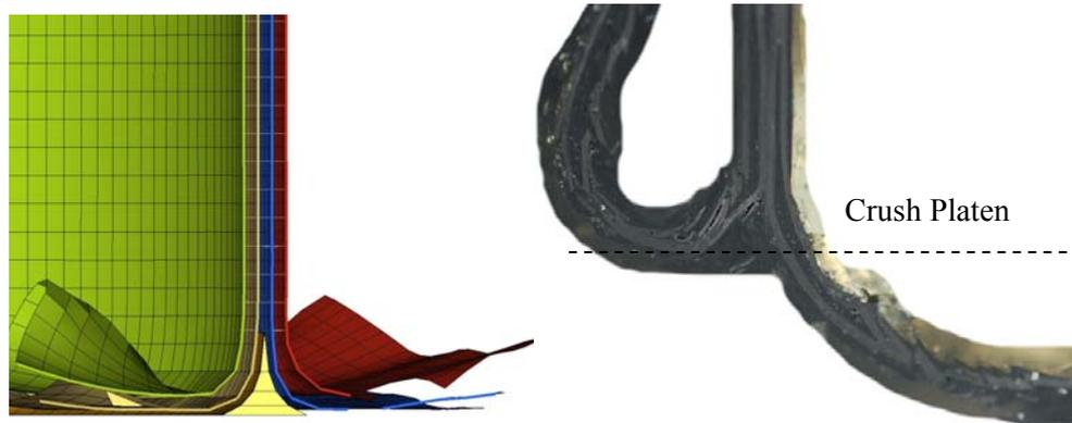
Figure 7.8. Images of simulated (left) and experimental (right) crush zones from Toray flat-platen tube crush tests.
