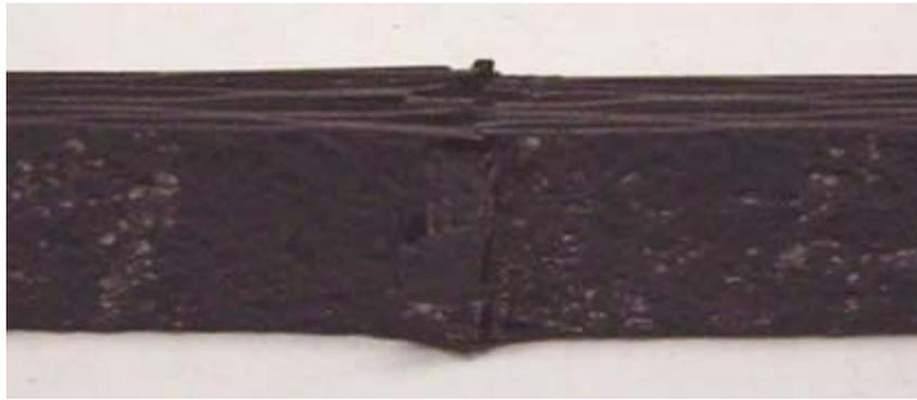
Figure 3.4. Failed specimen from in-plane compression testing.
