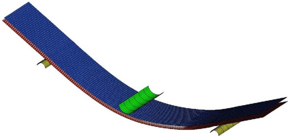
Figure 6.10. Image of CFRM ENF test underway.
