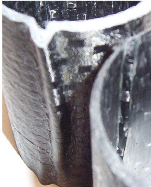
Figure 4.14. Image of large defect produced in preliminary process development. This ridge did not affect the energy absorption capability of the tube nor the behaviour.
