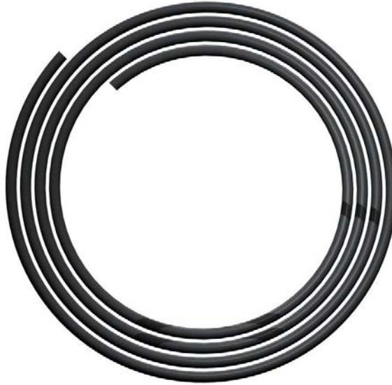
Figure 4.3. 'Swiss roll' lay-up produced by wrapping a single layer of material onto the mandrel.
