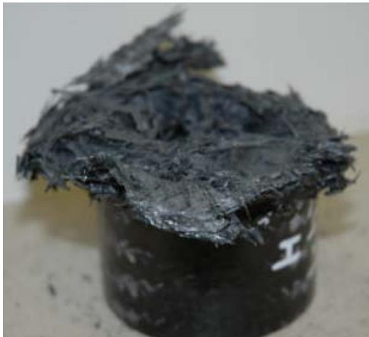
Figure 4.25. Failure mode observed in TFO-4 showing the transverse shearing failure mode.
