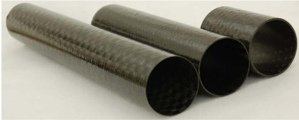
Figure 4.16. Image of 3 tubes of various fibre-forms showing the surface finish and product quality. (L-R: 2-layer [0°/90°] plain weave, 3 layer [±45°] 2x2 twill, 4 layer [0°/90°] 2x2 twill)
