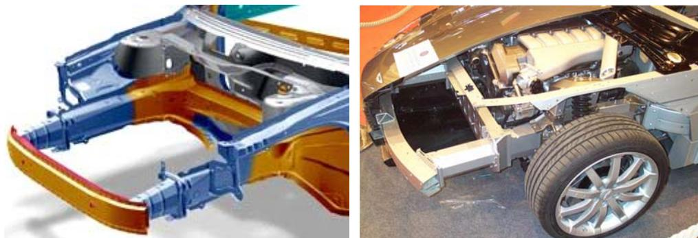
Figure 2.2. Two images of the frontal structures in different modern vehicles showing the bumper support, chassis rails and firewall. (left image taken from [www.sweden.se](http://www.sweden.se) – right photo taken by M.Silcock at JEC Expo, Paris, 2005)
