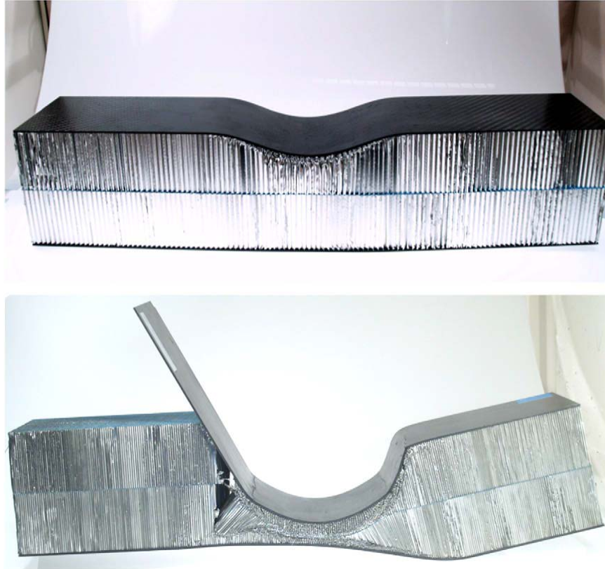
Figure 31. Partially crushed morphology of the assembly (top), the test was interrupted to take the picture. Final morphology of the assembly after testing (bottom).
