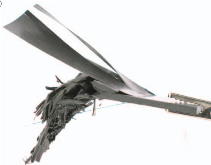
Figure 18. (a, b). Crushed specimen at 0 in. (0 mm) unsupported height (same as original NASA fixture), material B, and steeple trigger.
