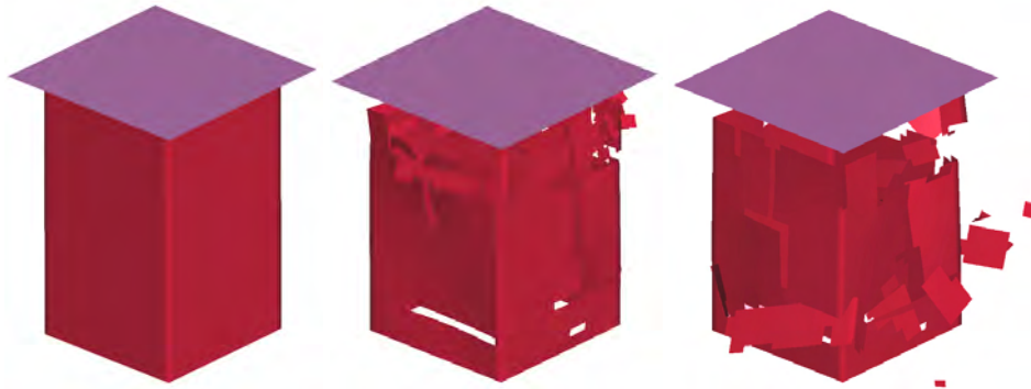
Figure 12. Example of an unstable crushing of the tubular shape with \text{SOFT}=0.64 Buckling starts after 2.446 millsec at a displacement of 0.3669 inches.
