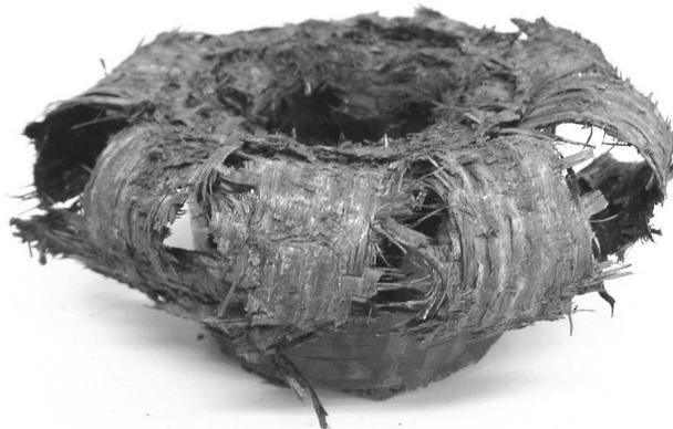
**Figure 5.** An example of the splaying mode of progressive failure observed in compression testing of TFO-0.
