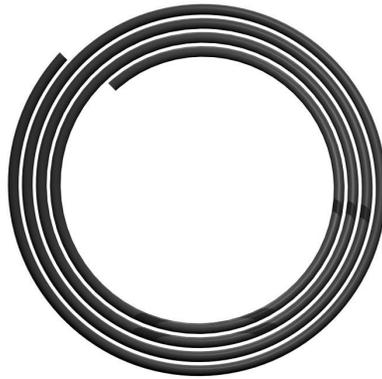
**Figure 2.** Schematic of typical 'swiss roll' lay-up produced when prepreg is wrapped onto mandrel.
